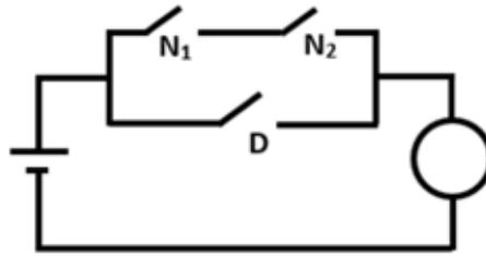
Q4. (i) In addition to having all of the switches closed, what other combinations of closed switches will turn on the bulb?
