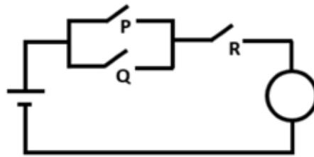
Q3. (i) Which switch must **always** be closed for the bulb to light?
