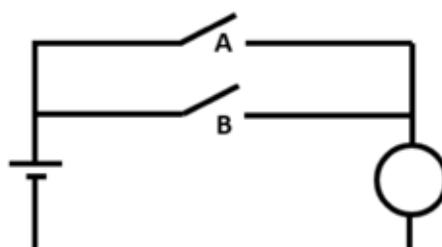
Q2. Now switch A and switch B are said to be *in parallel*. Using a logic operator, describe when the bulb will light up in Circuit 2.
